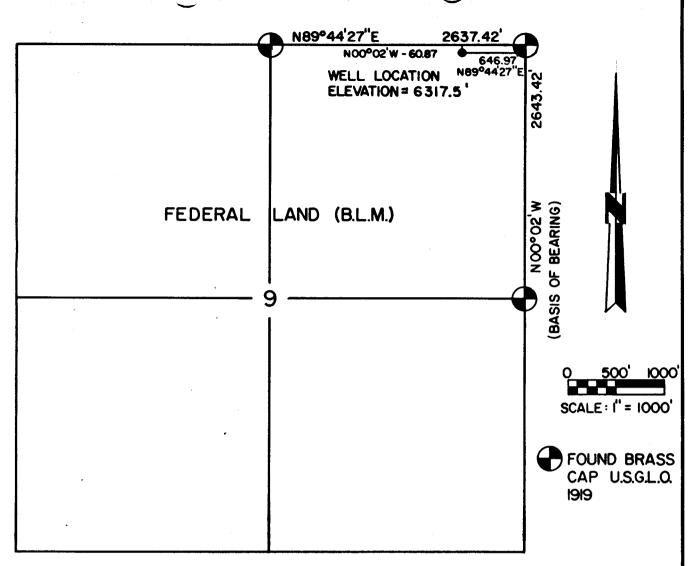
NOTE: The well location is 60.87 feet South of the North Section Line and 646.97 feet West of the East Section Line of the NE 1/4 of Section 9.
