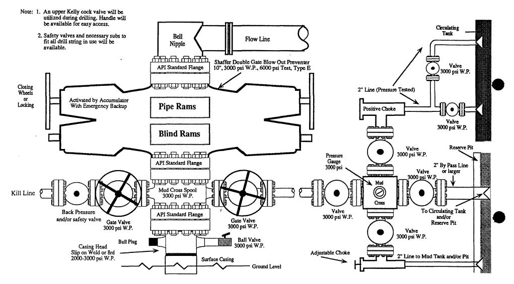
Note: This equipment is designed to meet requirements for a 2-M rating standard per 43 CFR part 3160 (amended). Proper operation and testing of equipment will be carried out per standard. 2,000 psi equipment can be substituted in the drawing to meet minimum requirements per standard.
